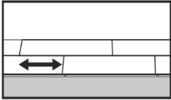
Fig 7. General distances between short ends. Minimum distance between short ends of planks in parallel rows shall not be less than 300-500 mm. This improves the stability of the floor.
